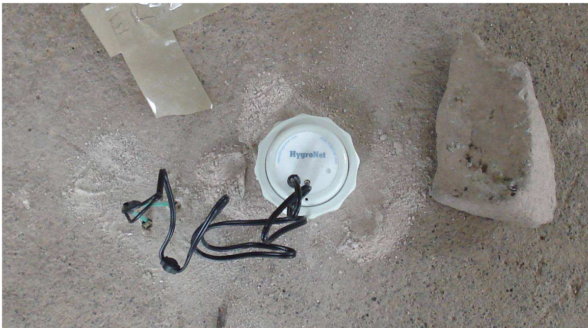
Fig 2:- Floor Probe Plan with WME probes taking reading at approx 70mm.
