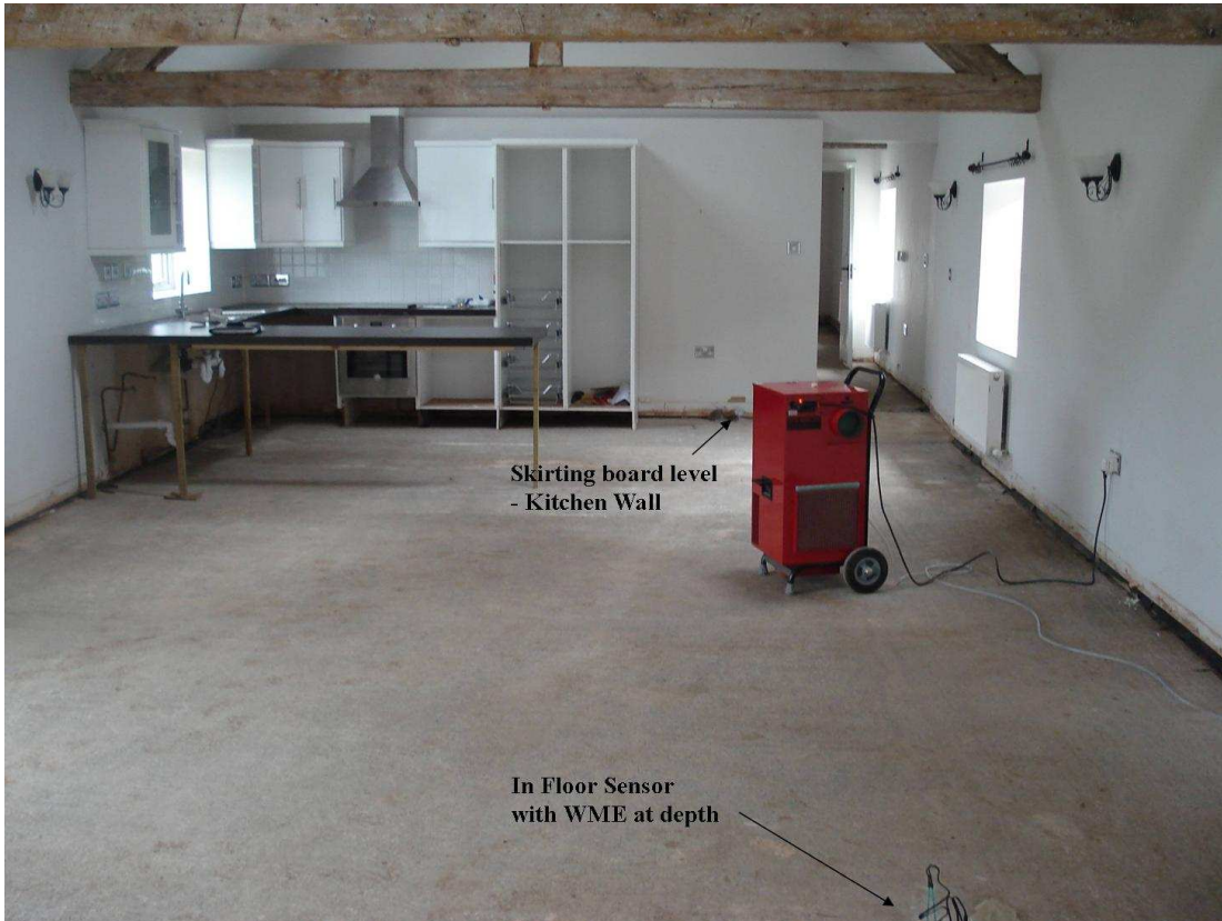
Fig 2:- Floor Probe Plan with WME probes taking reading at approx 70mm.
